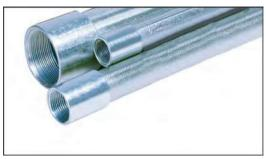
IMC is interchangeable with galvanized RSC. Both have threads with a ¾-inch-per-foot taper, use the same couplings and fittings, have the same support requirements and are permitted to be used in the same locations.
