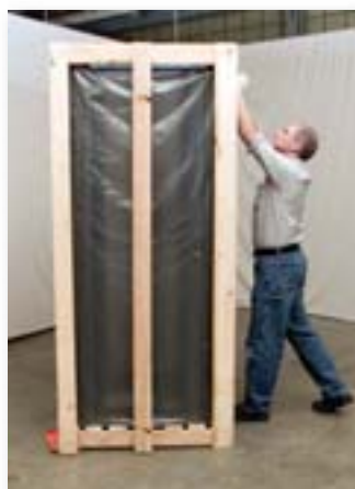
Cabinet enclosed in wooden frame to protect against all but the most severe impact.
