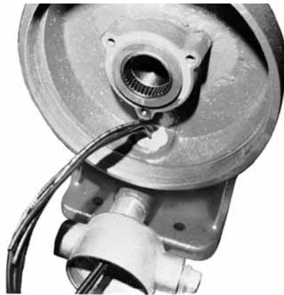
Fig. 3—Internal wiring showing factory-potted leads.
