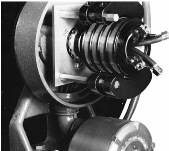
Fig. 4—Close-up view of external cast junction box for easy field installation.
